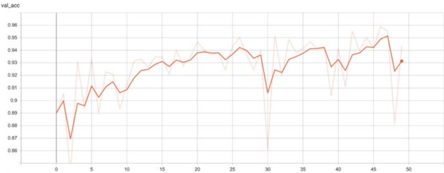
Fig. 21.8 Progression of the VGG16 validation accuracy after regularization
